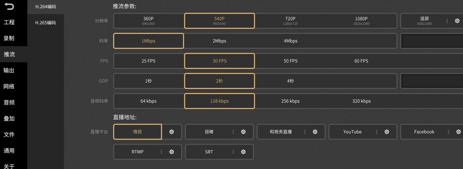
The screenshot displays the software's configuration menu for streaming. The left sidebar contains options: 工程 (Project), 录制 (Recording), 推流 (Streaming), 输出 (Output), 网络 (Network), 音频 (Audio), 叠加 (Overlay), 文件 (File), 通用 (General), and 关于 (About). The main area is titled 'H.264编码' (H.264 Encoding) and 'H.265编码' (H.265 Encoding). Under '推流参数' (Streaming Parameters), various settings are shown in a grid:
